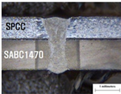
Fig. 4 Cross section of 590DP to SABC1470 combination.
