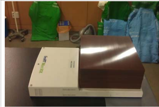
Fig. 2 The peripheral dose was measured by using solid phantom with mapcheck
