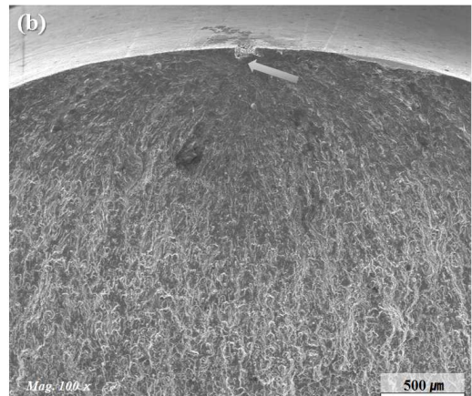
(b) Un-peened and corroded for 4 weeks
