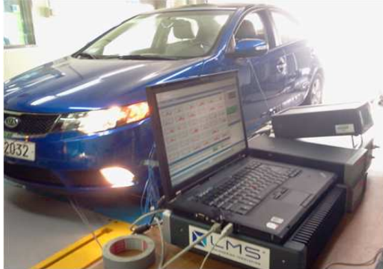
Fig. 4 Experiment set-up for identification of vibration path in Gamma gasoline direct injection (GDI) Engine
