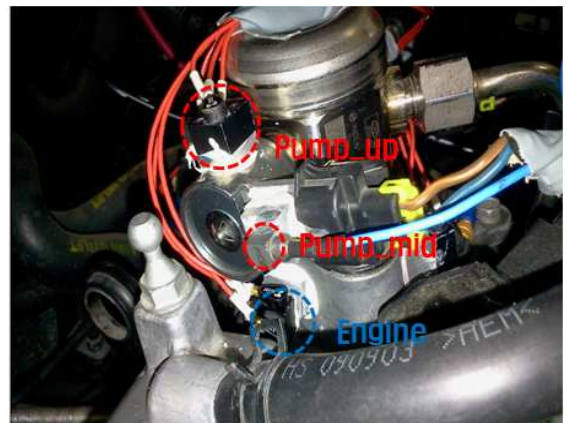
Fig. 7 Position of sensors for measurement of pressure pump vibration
