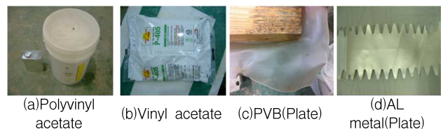
Figure 1. Using Adhesive materials
