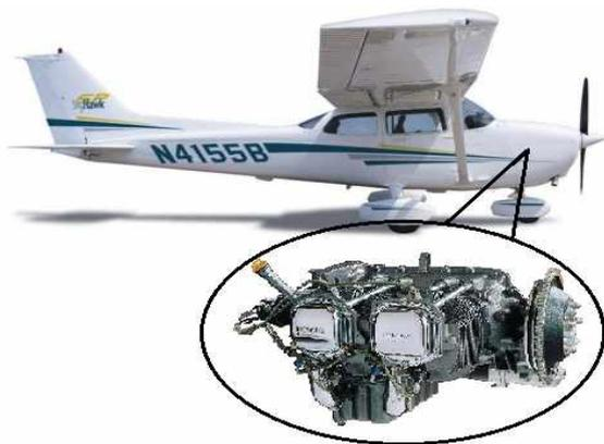
Fig. 11. Cessna 172 and O-360 engine
