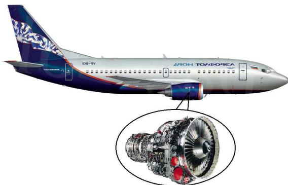
Fig. 12 B-737 and CFM56 engine
