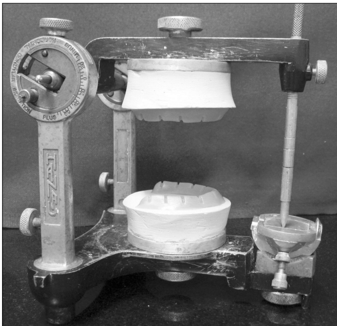
Fig. 5. Customized mounting platforms secured on articulator.
