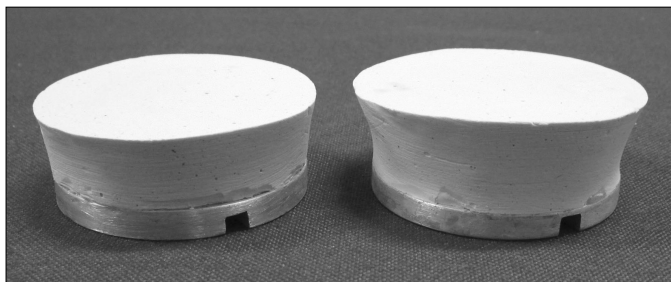
Fig. 2. Dental plaster poured in boxed mounting plates.
