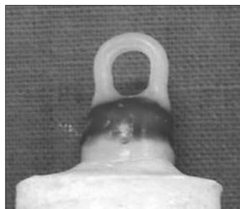
Fig. 3. Numbered and finished wax pattern.
