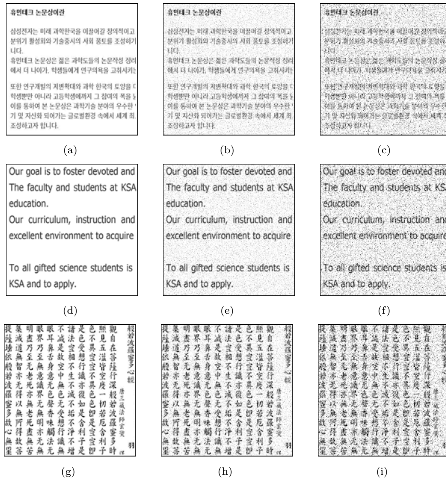
Figure 4.2. Test images used for experiments: (a) Korean image, (b) Noisy Korean image ( \sigma^2 = 0.01 ), (c) Noisy Korean image ( \sigma^2 = 0.05 ), (d) English image, (e) Noisy English image ( \sigma^2 = 0.01 ), (f) Noisy English image ( \sigma^2 = 0.05 ), (g) Chinese character image, (h) Noisy Chinese character image ( \sigma^2 = 0.01 ), (i) Noisy Chinese character image ( \sigma^2 = 0.05 )
