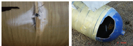
Fig. 2 Failures of composite layer and dome part in the vessel
