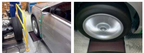
Fig. 15 Photo explanation for the rolling cleat test to measure the sound pressure in a vehicle
