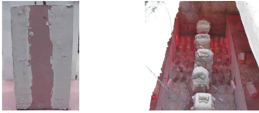
i) Model column ii) Fire resistance test Figure 2. Model structure and fire resistance test
