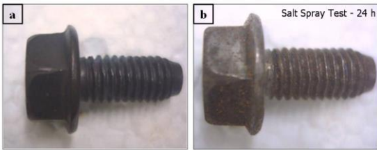
Fig.10 Pictures of Zn-Ni electrodeposited, and dipped in NaOH and Ni electroless deposited for 120 seconds and Cr coated bolt with two times top coating (1st Inorganic: 30sec/ 2nd Inorganic: 30sec): a) before and b) after salt spray test
