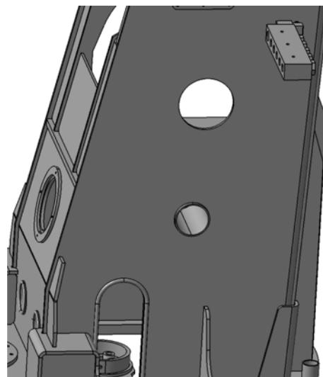
**Fig. 6** Interference of hose route
