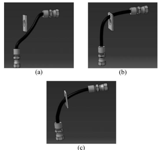
Fig. 10 Hose routing path : (a) Initial hose routing path, (b) Hose routing path using energy minimization (c) Modified hose routing path using target point
