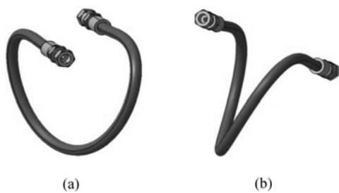
**Fig. 4** Form of hose route may differ depending on the plane chosen in CAD tool
