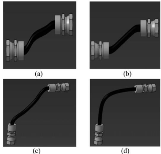
Fig. 8 Hose routing path : (a) Initial hose routing path, (b) Hose routing path using energy minimization, (c) Initial hose routing path, (d) Hose routing path using energy
