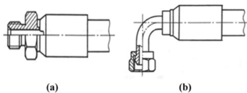
Fig. 2 Type of fitting : (a) Straight Type, (b) Elbow Type
