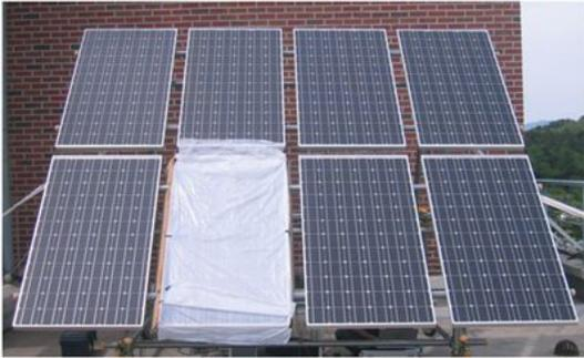
Fig. 6 Photo of PV string in experiment
