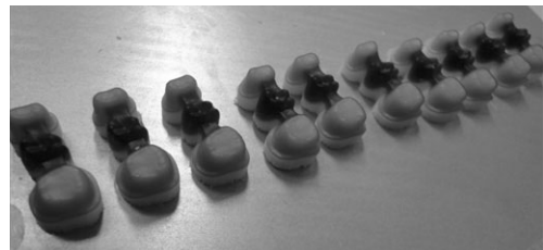
Fig. 3. Photopolymer 3 unit FDPs by rapid prototyping technique (3D printing technique)
