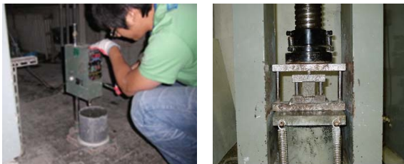
(a) Setting time check (b) Compressive strength test Fig 1. Test set up
