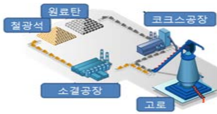
Blast furnace process
