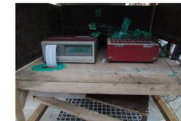
Photo 2. Refrigeration chamber container for curing of test specimen and measuring with data logger
