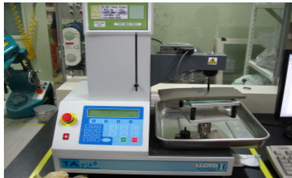
Fig.16 Test of surface hardness
