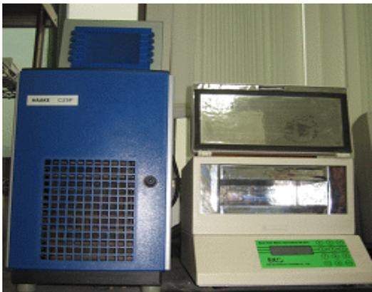
Fig. 3. Thermal conductivity measuring instrument
