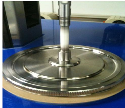
Fig 3. DSR(Dynamic Shear Rheometer); upper(25mm) and lower plate
