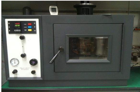
Fig. 3 RTFO(Rolling Thin Film Oven) Tester
