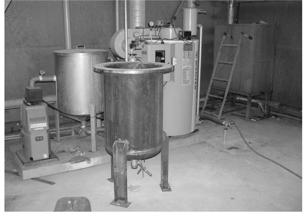
Fig. 1. Acid/alkali hydrolysis apparatus of animal cadavers.
