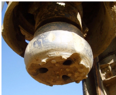
Fig. 2. Hammer drill used for sinking a pumping well (fore-end of barber drill).
