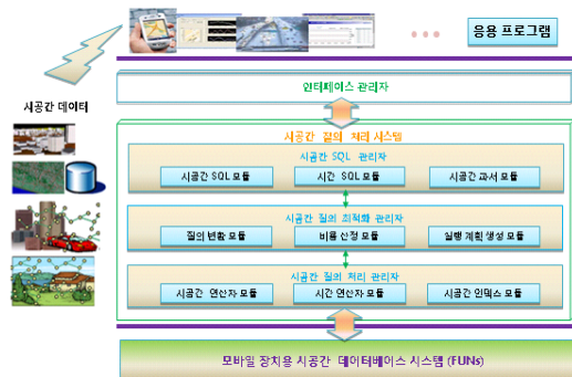
Figure 3. An architecture of spatio-temporal query processing system
