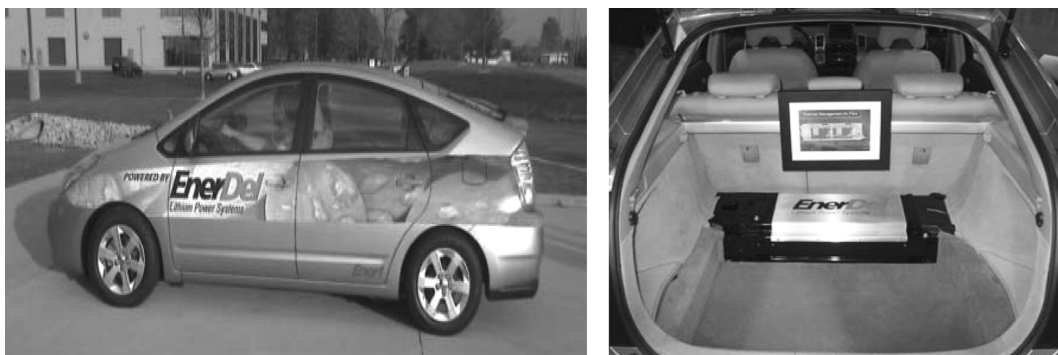
Figure 1. EnerDel/Argonne Advanced High-Power Lithium-Ion Battery (MS-TiO 2 system).
