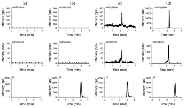
**Figure 2.** Representative MRM chromatograms of amitriptyline, nortriptyline and the IS in (a) SD rat blank plasma, (b) SD rat blank plasma spiked with LOQ (0.1 ng/mL for amitriptyline and 0.08 ng/mL for nortriptyline) with the IS, and (d) SD rat blank plasma with mid-concentration (10 ng/mL) analytes and the IS.
