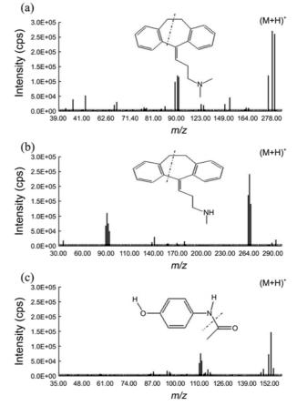
**Figure 1.** Tandem mass spectra showing ions from (a) amitriptyline, (b) nortriptyline, (c) acetaminophen (internal standard, IS) using electrospray ionization in positive ion mode.
