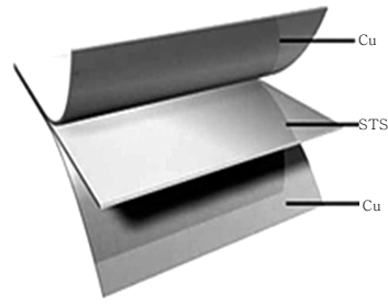
Fig. 1 Cross sectional structure of suggested clad metal lead frame materials.
