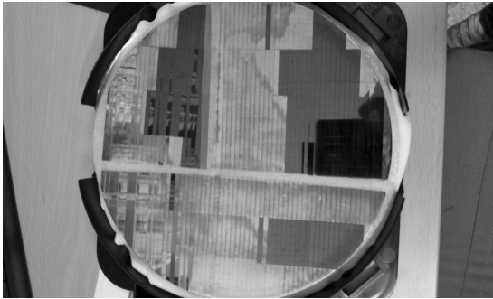
Fig. 5 Cu-Cu bonding wafer image after dicing process
