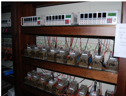
Fig. 4. Appearance of concrete specimens with CR-1212 power supply unit.
