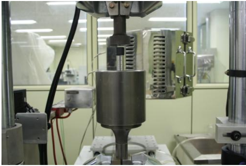
Fig. 3 Experimental set-up for closed-die compaction tests
