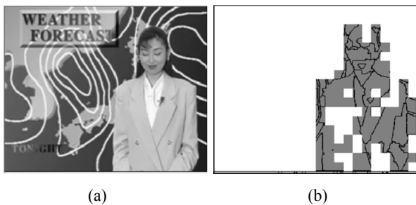
Fig. 10. The region that requires updated watershed segmentation (a) 4th frame of Weather sequence, (b) Updating region indicated by shaded blocks.
