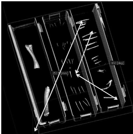
**Fig. 4.** Location & orientation. If the reference point is given, the distance and angle to the target fish bone can be measured. The orientation how the bone is located three dimensionally can be displayed visually (Virtual rendering image is used. The white arrows show distance and angle).
