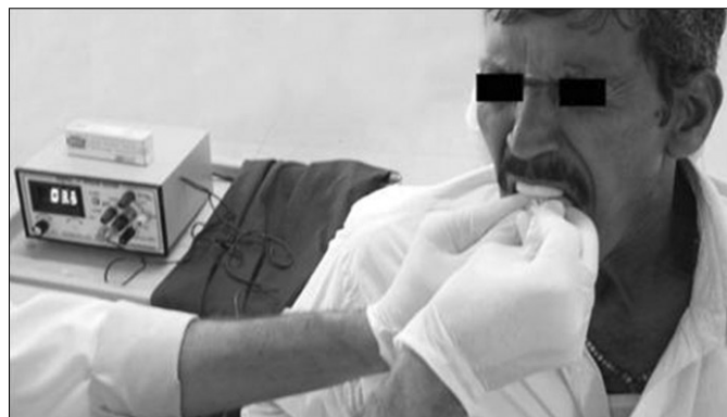
Fig. 6. Patient biting on the load cell of pressure transducer system.
