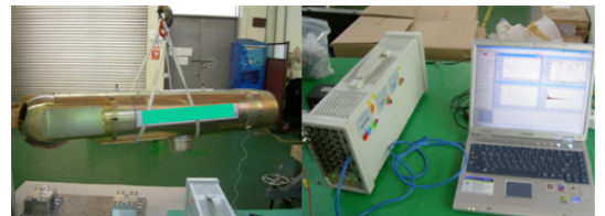
Fig. 6 Free-free modal test set-up
