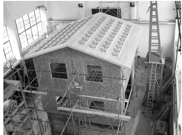
Fig. 2. Two-story wood frame specimen
