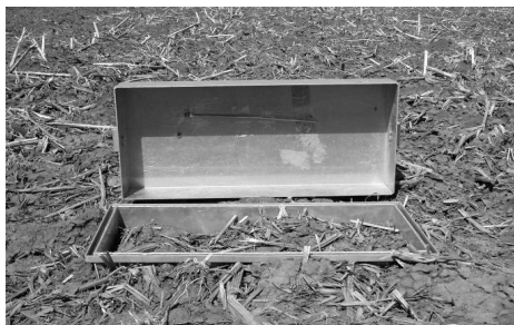
Fig. 2. Picture of anchor and chamber to collect GHG emitted from soil.
