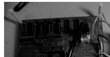
Fig. 12. Analog circuit implementation of PI controller.
