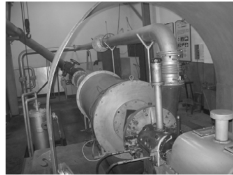
Fig. 13 Test bench of the centrifugal compressor
