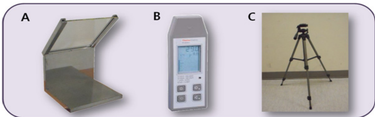
Fig. 1. The device was used digital survey-meter, L-Block lead glass shield and Holder. L-Block lead glass shield (Pb 6 mm) (A). Digital surveymeter is FH-40 (Thermo Scientific, USA) (B). Holder (HE-211, HAKUBA) (C).
