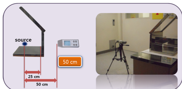
Fig. 3. Radiation were measured in the distance at 50 cm. Distance was 25 cm from source to radiation shield and 50 cm from source to digital surveymeter.
