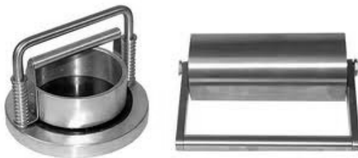
Fig. 2. Cobb sizing tester: (a) left – testing apparatus, (b) right - couch roll.
