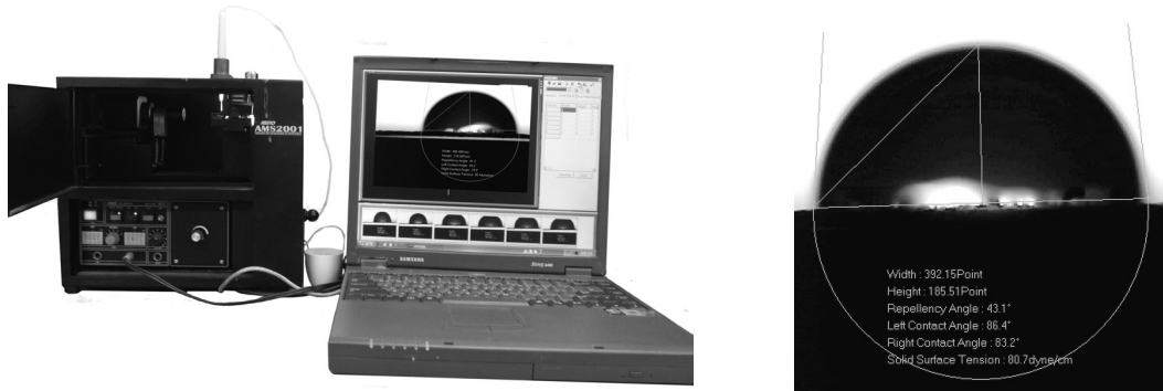
Fig. 4. Contact angle tester and the image of a liquid droplet.
