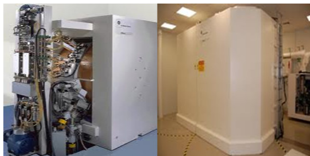
Fig. 2. PETTrace of GE Cyclotron.
