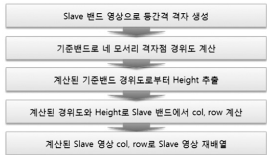
Fig 6. Terrain Relief Correction Procedure
