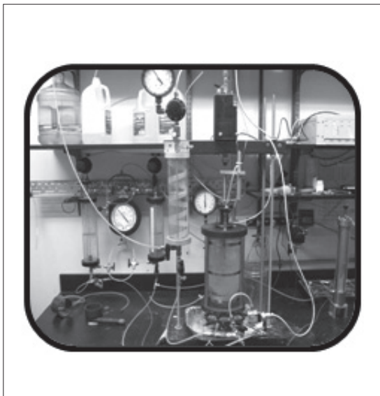
Fig. 9 Flow pump permeameter system: (a) Picture; (b) Schematic (Lee, 2011)
