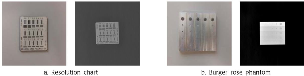
Fig. 1. Phantom for image evaluation at Humerus examination
