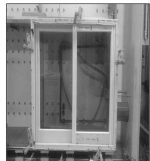
Fig. 2 Test body of Aluminum sash.
