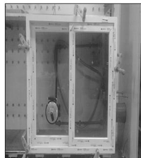
Fig. 1 Test body of Synthetic resins sash.
