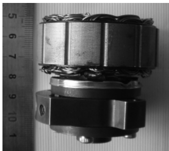
(a) Compressing and motor module
