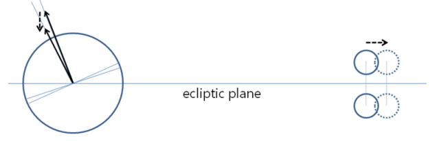
Fig. 2. — Schematic figure of the Earth-Moon system. The Earth's spin angular momentum decrease is accompanied with recession of the Moon, increase of the Earth's obliquity, and decrease of the lunar inclination to the ecliptic.
