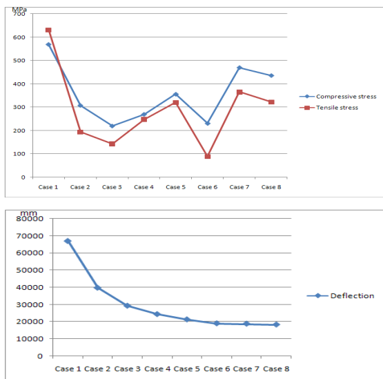
Fig. 5 Max stresses (tensile and compressive) and top deflection versus lay-up ratio (w/o core).
