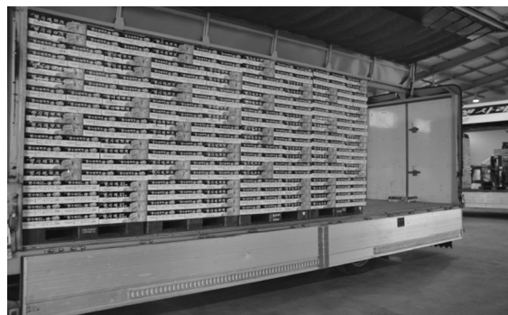
Figure 3. Real transportation test to verify the developed regression model for estimating the loss in compression strength of corrugated fiberboard containers.
